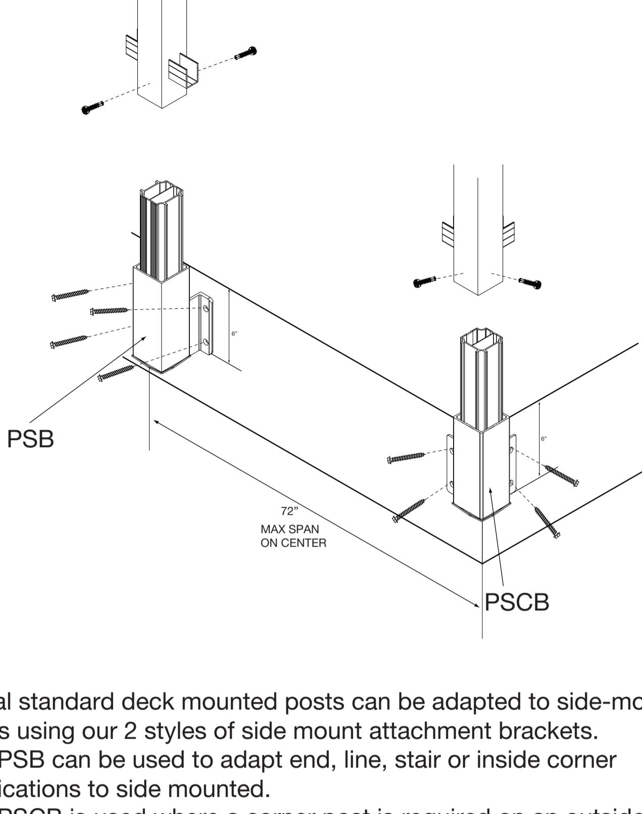
Regal standard deck mounted posts can be adapted to side-mounted posts using our 2 styles of side mount attachment brackets.
