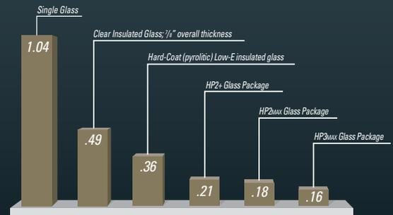
The lower the U-Factor the greater the insulation value. R-Value is the inverse (R=1/U) of the U-Factor. Center of glass factors calculated per Windows 5.2 simulation software (LBNL - Lawrence Berkeley National Laboratories).
