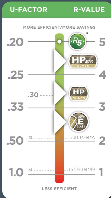
The lower the U-Factor, the greater the insulation value. R-Value is the inverse ( $R=1/U$ ) of the U-Factor. Total Unit Factors determined per NFRC-100 (National Fenestration Rating Council). Chart shows relationship between performance and Ply Gem Windows glass package options, not including energy package upgrade.
