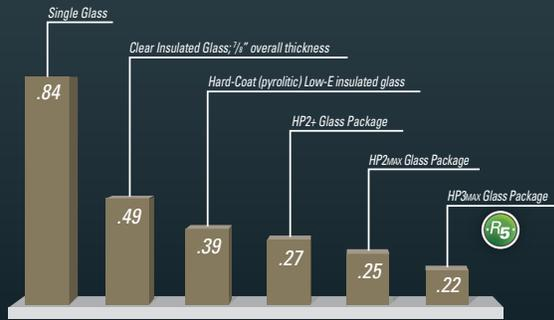
The lower the U-Factor the greater the insulation value. R-Value is the inverse (R=1/U) of the U-Factor. Total Unit Factors determined per NFRC-100 (National Fenestration Rating Council). The HP glazing option is certified to NFRC-100, and Hi R+Plus meets all ENERGY STAR requirements. Based on double hung product style.
