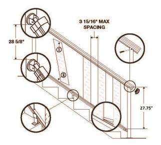
Installing ILSP(in-line stair post) at bottom of stairs. Begin by mounting the bottom stair post on the bottom tread of the stairs. The post should be mounted
