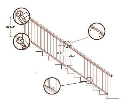
Installing ILSP(in-line stair post) as a mid post and using connecting splice. When installing longer stair runs or when conncting the rails using the connecting splice, a mid post be required. A top rail splice can be used to join top rails in order to accommodate longer stair runs.
