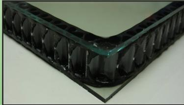
**Duralite warm edge spacer** along with **Soft Coat Low E** on surface 2 and **Triple Silver Hard Coat** on surface 4, plus concentrated argon gas, allow us to reach R5 without Triple Glazing!
